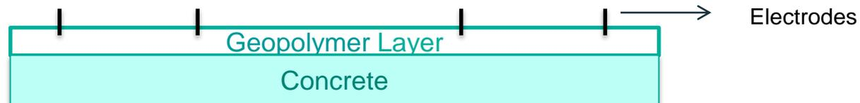
Figure 8 – Scheme of geopolymer layer put on a concrete samples, with electrodes embedded.
