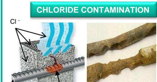
The diagram shows a steel rebar in concrete with Cl<sup>-</sup> ions penetrating. 'Corrosion products' are shown as orange and red particles on the rebar surface. The photo shows two pieces of steel rebar, one with significant pitting corrosion.
