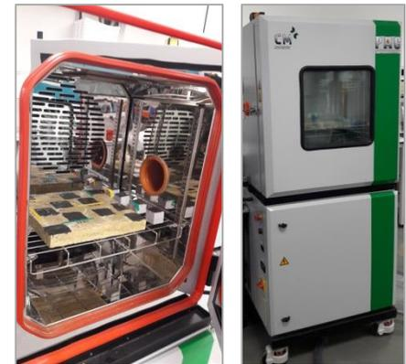
**Figure 11** – Samples in the Environmental chamber.
