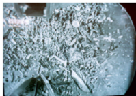
B - Magnox - Partially Corroded Swarf and Magnesium Hydroxide Sludge
