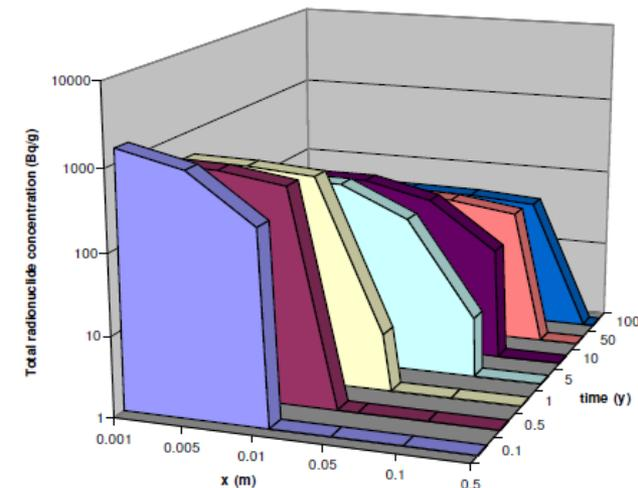
Figure 1. In-diffusion of contamination from the surface of a concrete slab (at the left side of the plot) after periods from 0.1 to 100 years.
