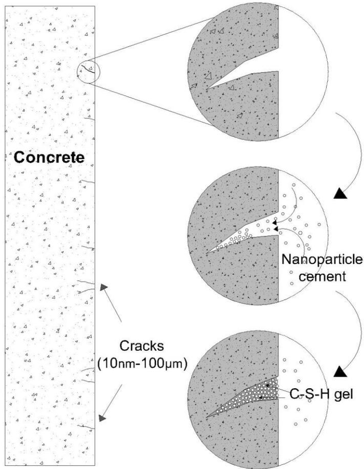
Aim of the project is to investigate new cement mixtures able to seal nano-cracks, preventing deterioration and giving an adequate (controlled) impermeability to existing concrete structures.
