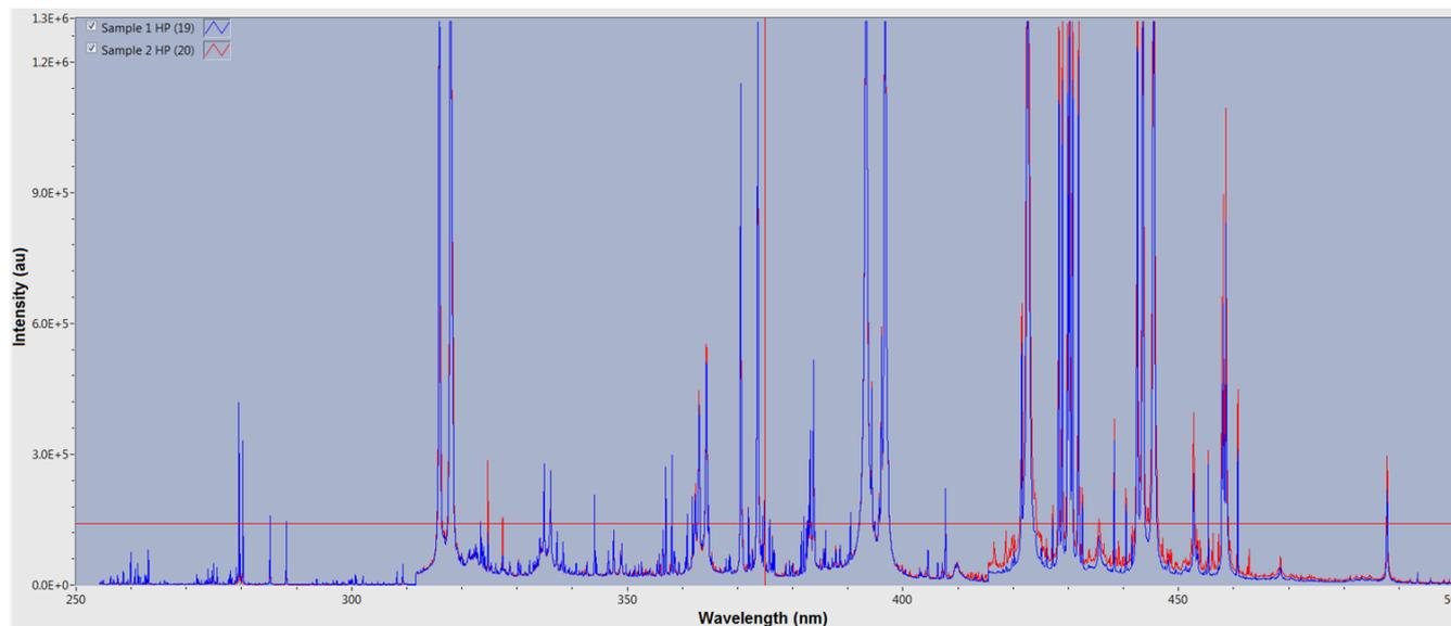
wavelength vs intensity plot for reference and 1% contaminated sample
