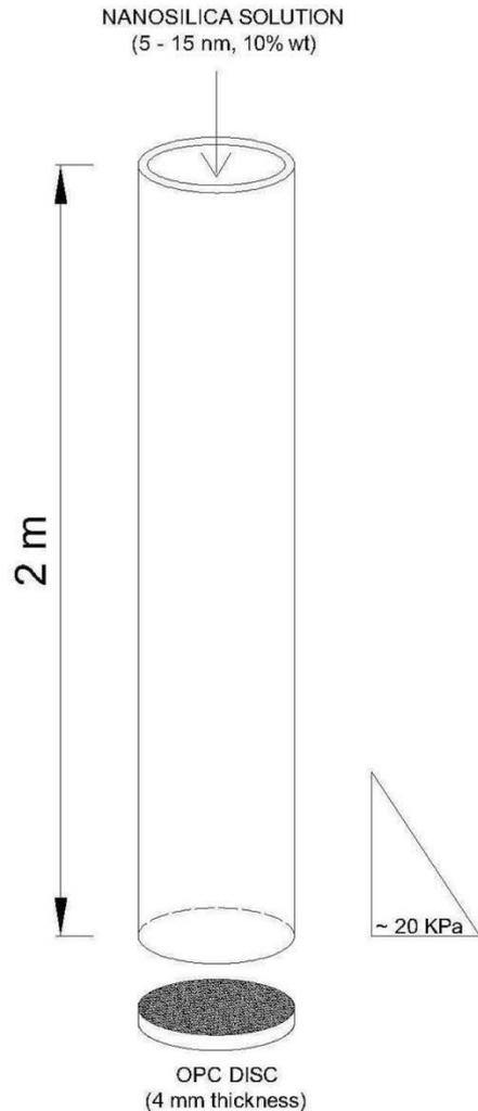
Low-pressure nanosilica injection was investigated at lab-scale. A solution of **nanosilica** (particle size range of 5 – 15 nm) will be injected through a *28 days cured OPC* disc (thickness 4 mm) at a ~ **20 kPa** of hydrostatic pressure.
