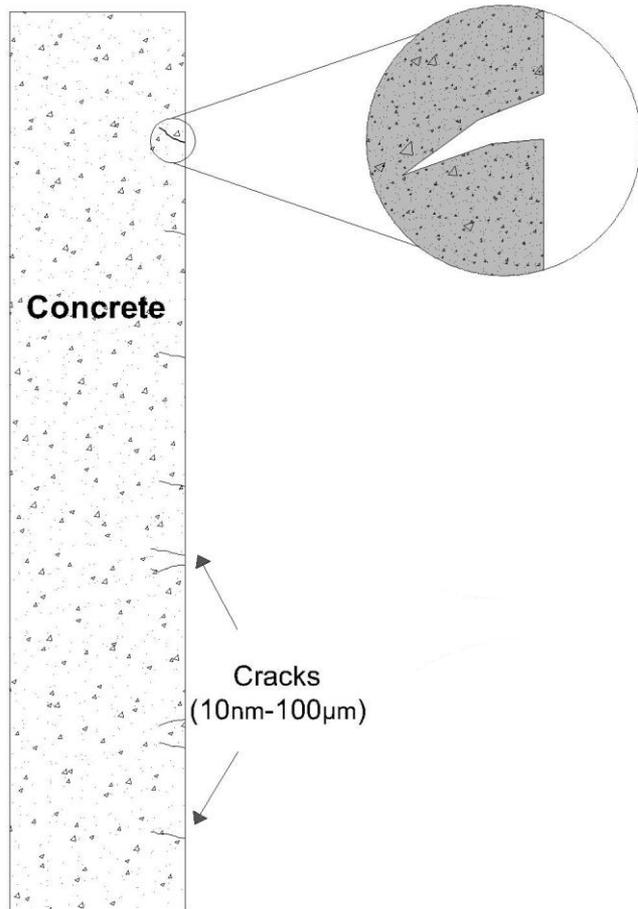
Aim of the project is to investigate new cement mixtures able to seal nano-cracks, preventing deterioration and giving an adequate (controlled) impermeability to existing concrete structures.
