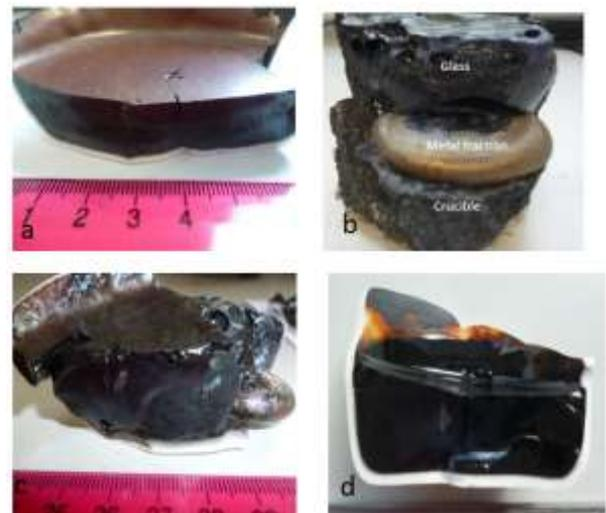
Fig6: Showing vitrified simulant PCM drum mock ups (a) PVC waste, (b) metal waste, (c) masonry waste, and (d) mixed waste
