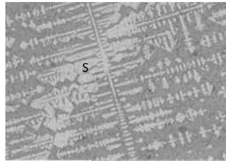
Fig9: BSE image showing microstructure of slag produced by vitrification of PVC waste type. S corresponds to identified spinel phase
