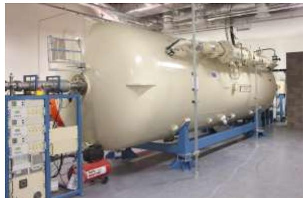
Figure 4 Dalton Cambrian Facility's 5MV Pelletron housed in the accelerator hall.
