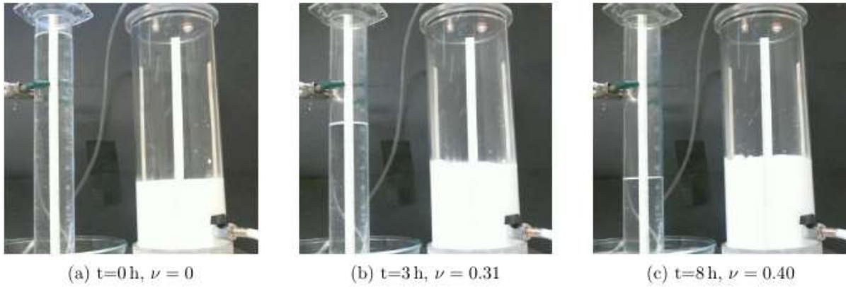
Figure 1: Bed swell due to gas retention in 8 Pa Mg(OH)<sub>2</sub> sludge
