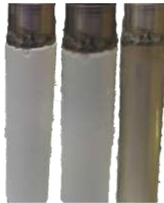
**Figure 7** Filter cake formed with no shear (left), low shear (middle) and high shear (right)
