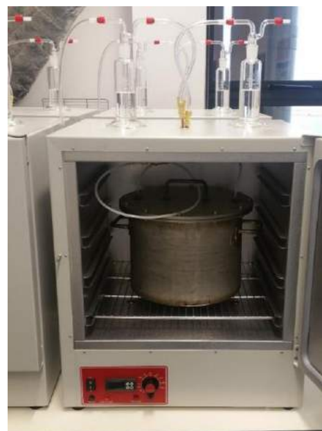
Fig 10: Controlled nitrogen atmospheric chamber to avoid carbonation of samples and ensure high PH conditions to simulate the GDF environment.
