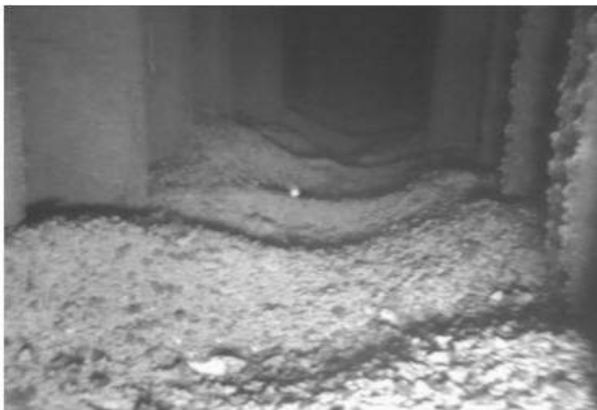
Figure 1 Radioactive sludge at the bottom of a long-term storage [10]
