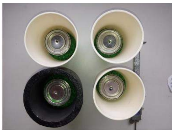
Fig5: Simulant waste with addition of glass frit at 1:1 wt ratio
