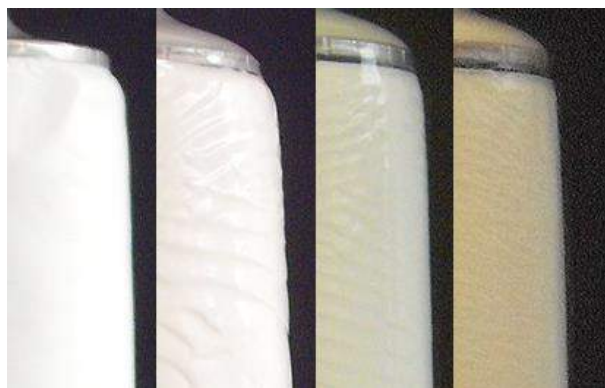
Figure 6, Filter cake formed with increasing shear left to right
