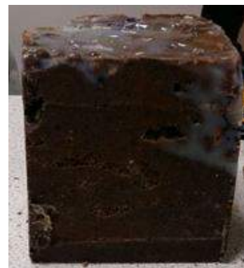
Figure 8 Colloidal silica grouted sample of initially loose soil.
