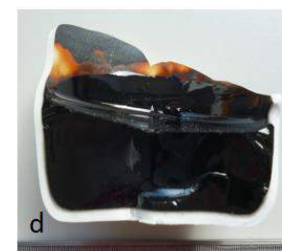
Fig6: Showing vitrified simulant PCM drum mock ups (a) PVC waste, (b) metal waste, (c) masonry waste, and (d) mixed waste
