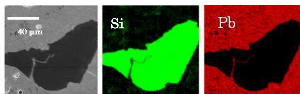
Figure 10. 10 wt.% waste loading PB EDS maps.
