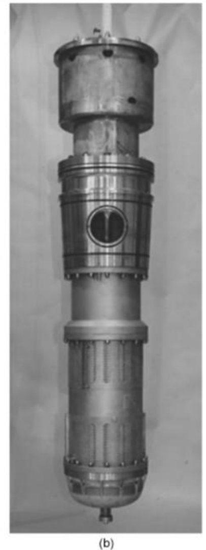
3.6 a and b Schematic representation and photograph of an EARP ultrafilter module. b Source: Nuclear Decommissioning Authority ("NDA"), copyright: Nuclear Decommissioning Authority ("NDA").
