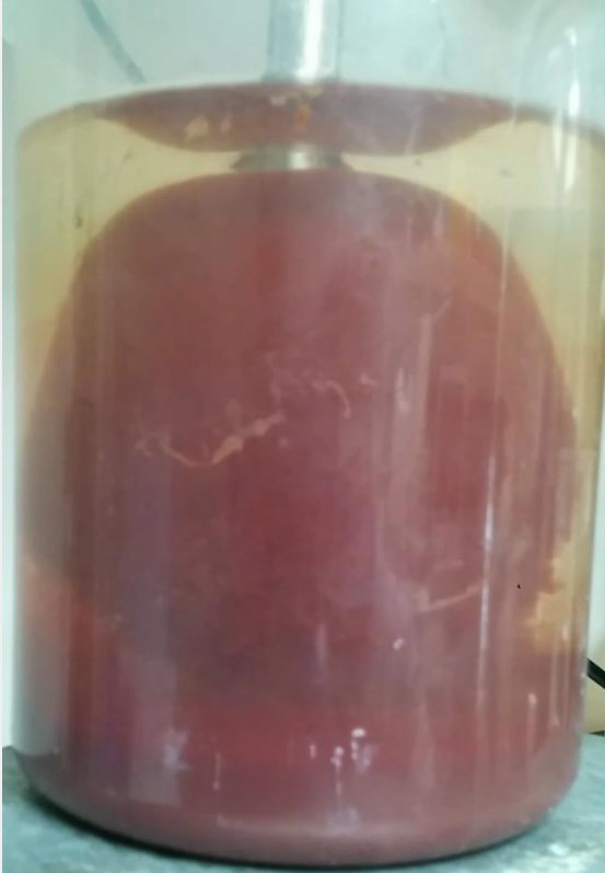
Cake formed on ceramic filter without shear before (left) and cutaway after being removed from water (middle)*
