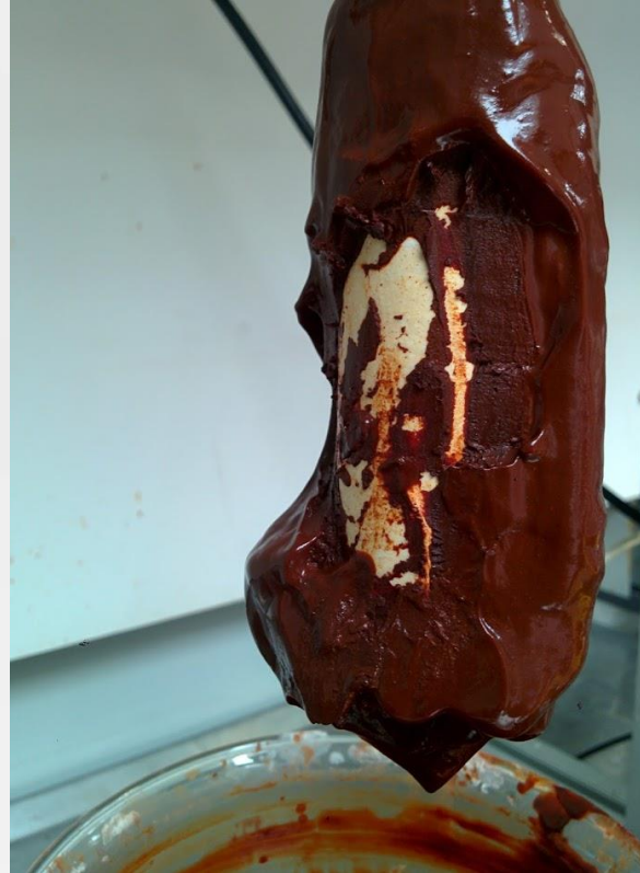
Cake formed on ceramic filter without shear before (left) and cutaway after being removed from water (middle)*
